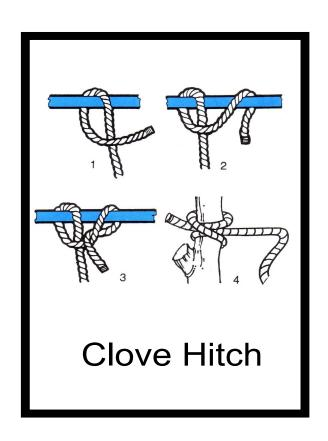
A clove hitch is used to connect a small line to a larger rope or spar at right angles or for a two way guy during erection of poles and to fasten a rope to a spar while under strain. Also starts a square lashing.
